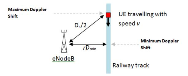
The expression  $D_s / 2$  is the initial distance of the train from eNodeB, and  $D_{\min}$  is the minimum distance between eNodeB and the railway track. Both variables are measured
