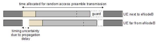
Therefore the size of the guard period determines the cell radius, as any propagation delay exceeding the guard time would cause the random access preamble to overlap the following subframe at the eNodeB receiver.
