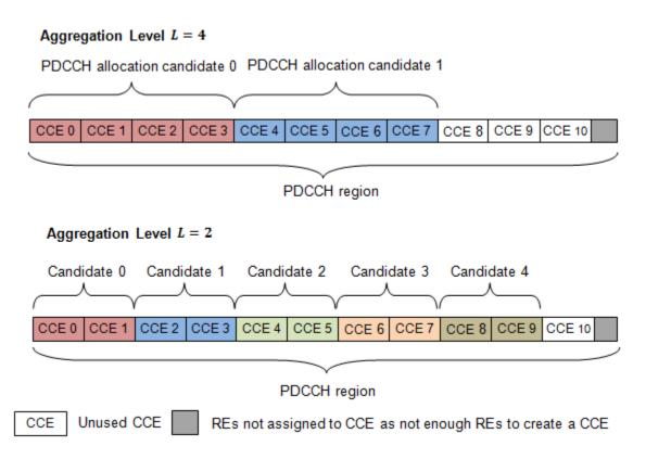
In this example, only 11 CCEs are available due to bandwidth constraints. The CCEs used to construct each PDCCH candidate are defined by the following equation.
