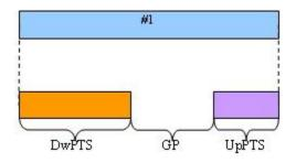
The lengths of DwPTS, GP, and UpPTS can take one of 10 combinations of values, termed special subframe configurations 0 through 9. The LTE standard, TS 36.211 Table 4.2-1, specifies the lengths in terms of the fundamental period of the OFDM modulation, but the lengths can be interpreted in terms of OFDM symbols as shown in the following table.
