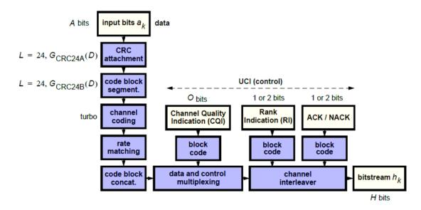
It is possible for the PUSCH to carry only control information and no data. In this case, only the control information coding and multiplexing chain are followed as per the preceding diagram.
