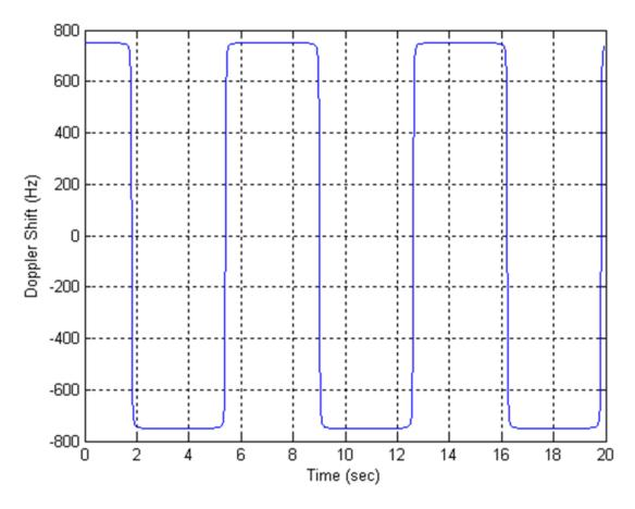
These parameters result in the Doppler shift, applied to all frequency bands, shown in the following figure.
