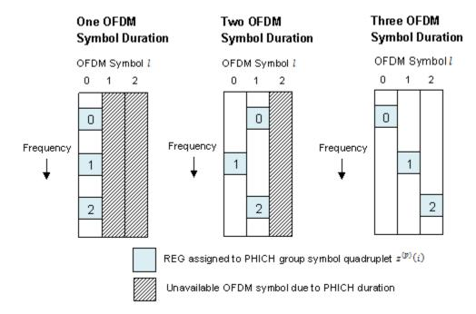
The subcarrier index,  $k'_i$ , of the REG is based upon the cell ID,  $N_{ID}^{cell}$ , and is chosen to spread the three symbol quadruplets over the entire bandwidth.
