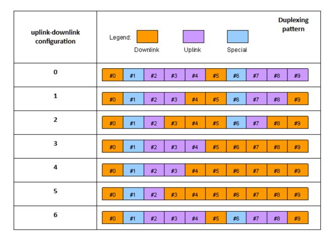
The special subframe (subframe 1 in every uplink-downlink configuration, and subframe 6 in uplink-downlink configurations 0, 1, 2 and 6) contains a portion of downlink transmission at the start of the subframe (the Downlink Pilot Time Slot, DwPTS), a portion of unused symbols in the middle of the subframe (the Guard Period) and a portion of uplink transmission at the end of the subframe (the Uplink Pilot Time Slot, UpPTS), as shown in the following figure.
