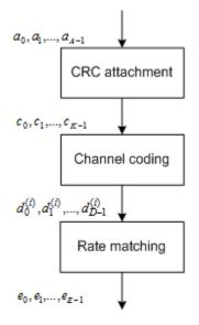
To form the PDCCH payload, the DCI undergoes coding as shown in the following figure.
