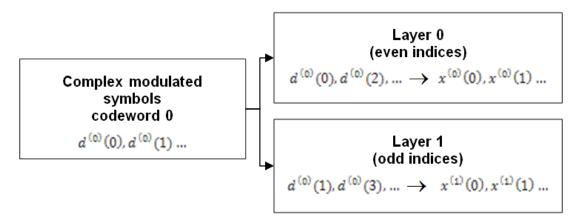
• **Two Codewords** — Codeword 0 is mapped to layer 0 and codeword 1 is mapped to layer 1, as shown in the following figure.
