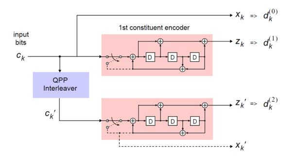
The output of the encoder is three streams,  $d_k^{(0)}$ ,  $d_k^{(1)}$ , and  $d_k^{(2)}$ , to achieve a code rate of 1/3.
