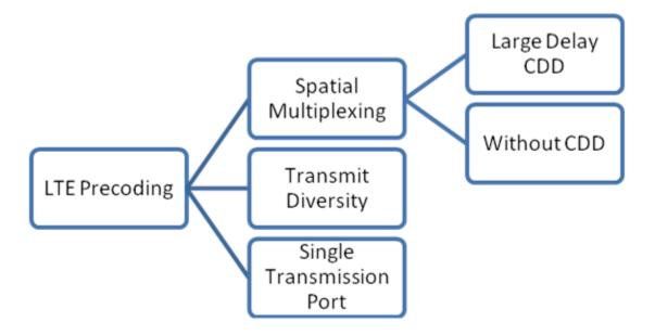
The precoder takes a block from the layer mapper,  $x^{(0)}(i), x^{(1)}(i), \dots, x^{(v-1)}(i)$ , and generates a sequence for each antenna port,  $y^{(p)}(i)$ . The variable p is the transmit antenna port number, and can assume values of  $\{0\}, \{0,1\}, \text{ or } \{0,1,2,3\}$ .
