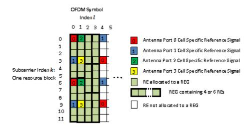
The REG allocation within the first OFDM symbol is the same as for a one or two antenna port configuration. Four cell specific reference signals are present in the second OFDM symbol therefore eight REs are available for the mapping of control data. The twelve REs are divided into two REGs, each containing six REs. The third and fourth OFDM symbols contain no reference signals so three REGs are available.
