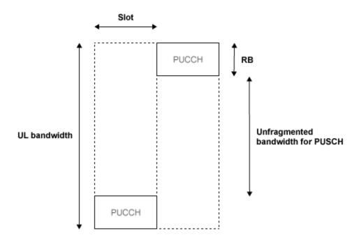
Bandwidth edges are used so that a large unfragmented portion of the spectrum remains to allocate to the PUSCH. If this spectrum was fragmented by multiple PUCCHs it would not be possible to allocate a number of contiguous RBs to a UE, hence the single carrier nature of SC-FDMA would be lost.
