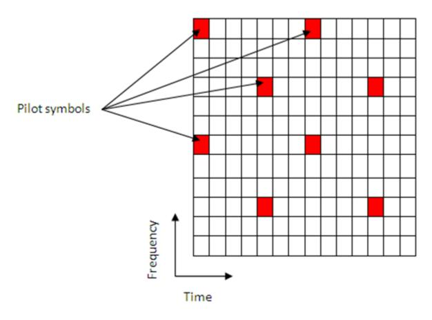
The unique positioning of the pilots ensures that they do not interfere with one another and can be used to provide a reliable estimate of the complex gains imparted onto each resource element within the transmitted grid by the propagation channel.
