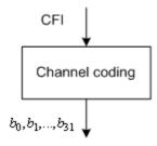
Using the following table contains the CFI codeword for each CFI value. Using these codewords corresponds to a block encoding rate of 1/16, changing a two bit CFI value to a 32 bit codeword.
