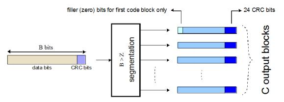
If no segmentation is needed, only one code block is produced. If B is less than the minimum size, filler bits (zeros) are added to the beginning of the code block to achieve a total of 40 bits.
