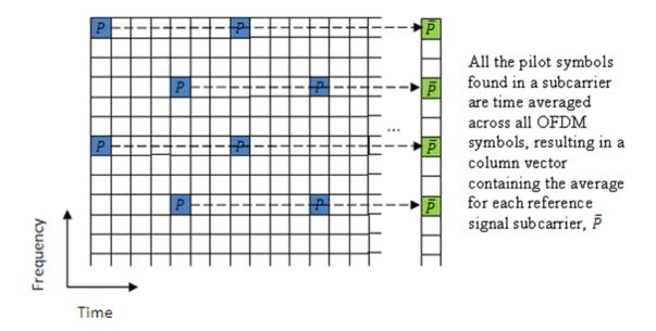
The averages of the pilot symbol subcarriers are then frequency averaged using a moving window of maximum size 19.
