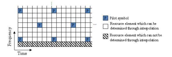
In this case, channel estimates at the edges cannot be interpolated from the pilot symbols. To overcome this problem, virtual pilot symbols are created. The function lteDLChannelEstimate creates virtual pilot symbols on all the edges of the received grid to allow cubic interpolation.
