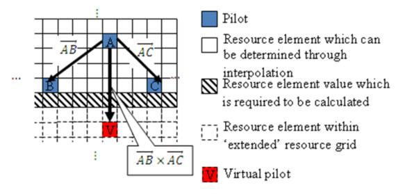
**Note:** Virtual pilots are only created for the  $MATLAB^{\text{(B)}}$  'linear' and 'cubic' interpolation methods.
