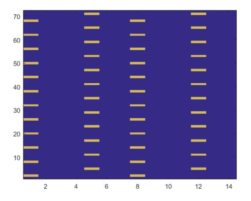
The resulting matrix has the complex symbols in <code>rsAnt0</code> and <code>rsAnt1</code> in the appropriate locations, specified by <code>indAnt0</code> and <code>indAnt1</code>.
