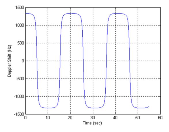
Both of these scenarios result in Doppler shifts that apply to all frequency bands. The Doppler shift trajectory for scenario 1 is shown in the following figure.
