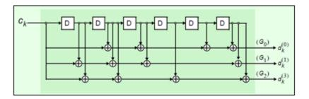
Each output stream of the coder is obtained by convolving the input with the impulse response of the encoder, as shown in the following equation.
