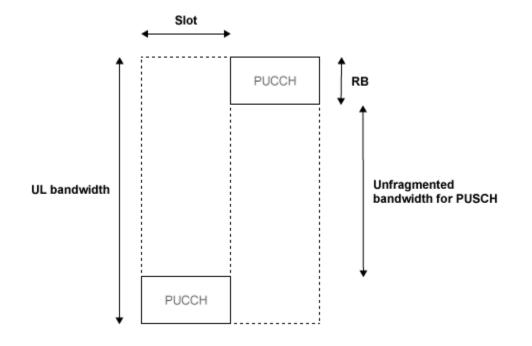
Bandwidth edges are used so that a large unfragmented portion of the spectrum remains to allocate to the PUSCH. If this spectrum was fragmented by multiple PUCCHs it would not be possible to allocate a number of contiguous RBs to a UE, hence the single carrier nature of SC-FDMA would be lost.
