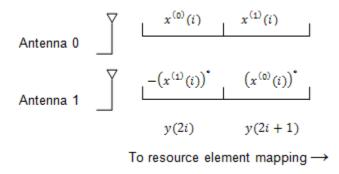
As any two columns in the precoding matrix are orthogonal, the two symbols,  $x^{(0)}(i)$  and  $x^{(1)}(i)$ , can be separated at the UE.
