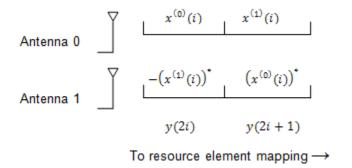
As any two columns in the precoding matrix are orthogonal, the two symbols,  $x^{(0)}(i)$  and  $x^{(1)}(i)$ , can be separated at the UE.
