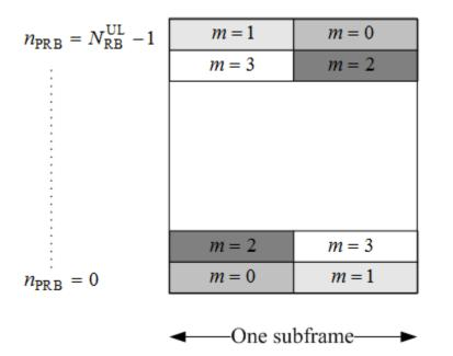
PUCCH formats 1, 1a, and 1b make use of four SC-FDMA symbols per slot. If normal cyclic prefix is used, the remaining 3 symbols, 2 for extended cyclic prefix, are used for PUCCH demodulation reference signal (DRS). If the sounding reference signal (SRS) overlaps the PUCCH symbols, only three symbols are used in the second slot of the subframe. The mapping of the symbols is illustrated in the following figure.
