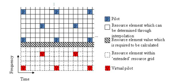
In this system, the resource grid is extended, with virtual pilot symbols created in locations which follow the original reference signal pattern. The presence of virtual pilot symbols allows the channel estimate at the resource elements, which previously could not be calculated by interpolation, to be calculated by interpolation using the original and virtual pilot symbols.
