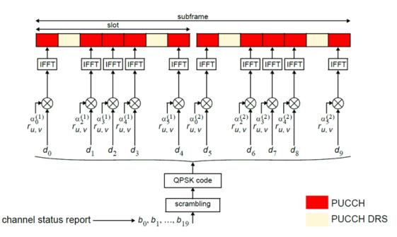
The cyclic shifted sequence applied to randomize intercell interference is denoted here by  $r_{u,v}$ . For extended cyclic prefix, where there are only six SC-FDMA symbols per slot, the mapping to resources changes slightly. In this case, only one reference signal is transmitted per slot, and the signal occupies the third symbol in each slot.
