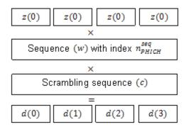
The variable w is an orthogonal scrambling sequence with index  $n_{PHICH}^{seq}$ . The sequences are given in the following table.
